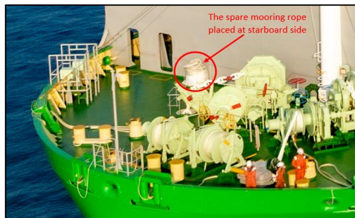
Figure 5 – The spare mooring rope placed at starboard side (Source: the Company, red annotations by TSIB)
